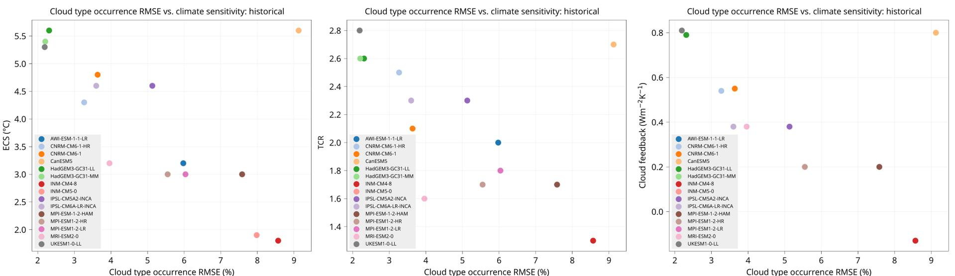
**Figure 3:** Dependence of model ECS, TCR and cloud feedback on the total cloud type occurrence root mean square error (RMSE) as shown in Figure 2.
