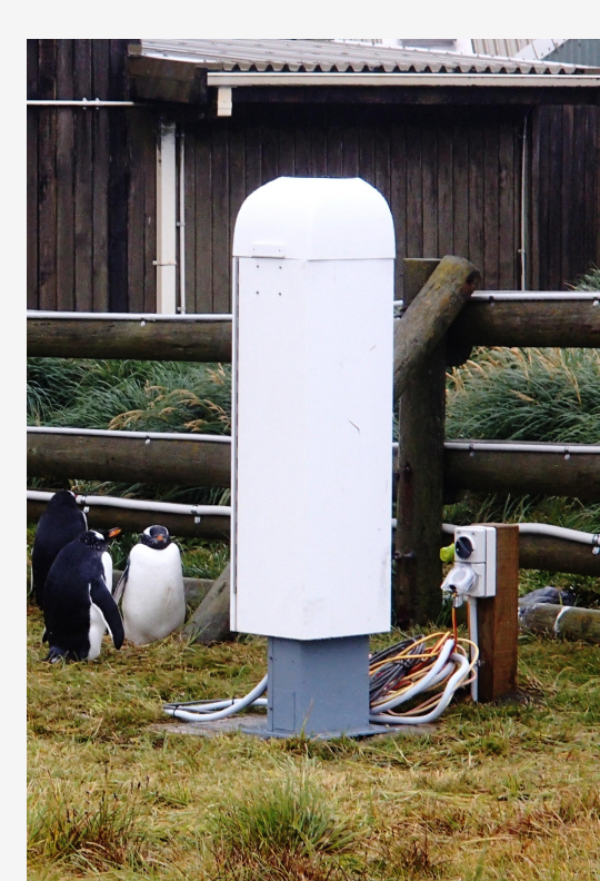
Figure A2 | Installation of Vaisala CL51 on Macquarie Island (2016).
