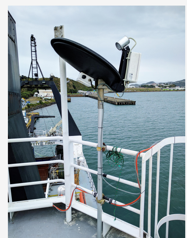
Figure A4 | Metek MRR-2 on RV Tangaroa in Wellington, en route to Campbell Plateau (2017).
