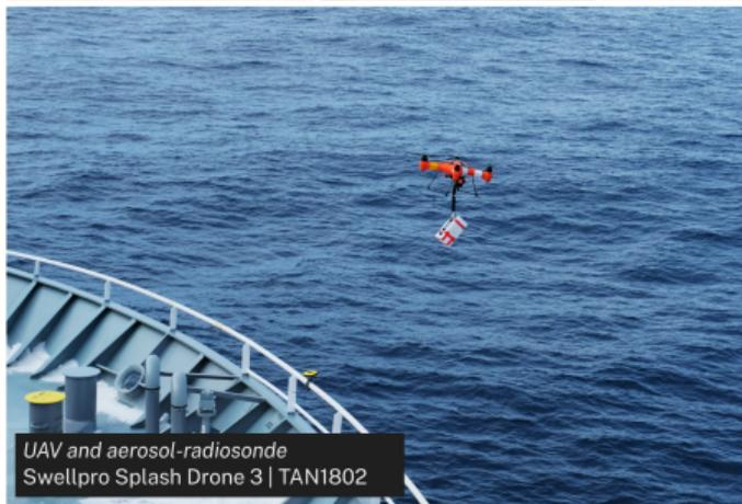
UAV and aerosol-radiosonde
